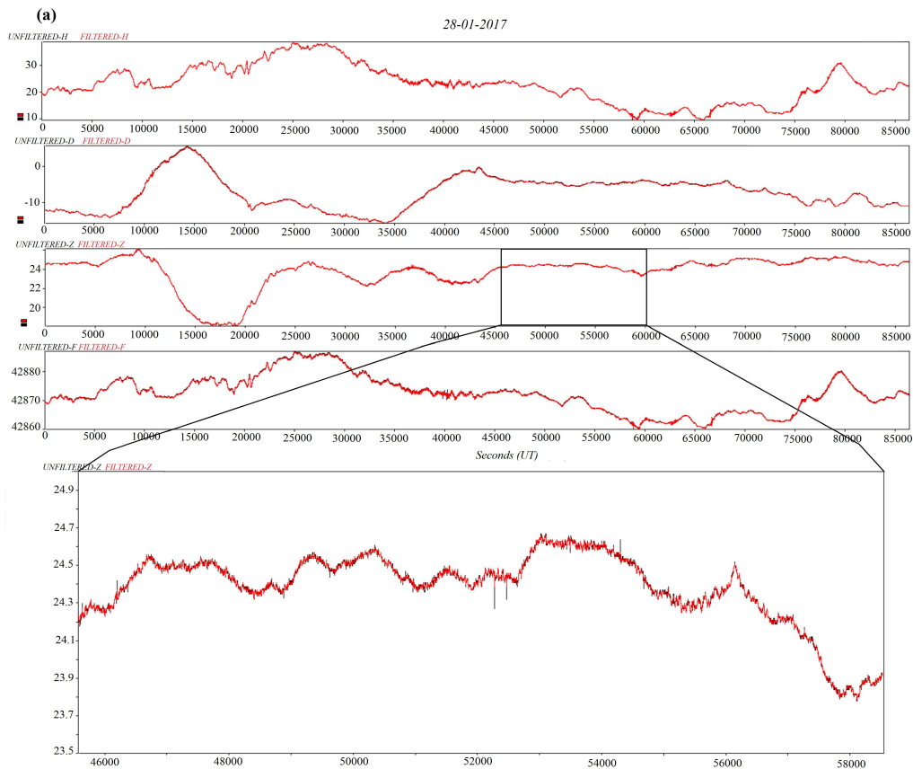
Fig. 4. Figure 9a. Sample plots of 1 second raw (black colour line) and filtered data (red colour line) with cut-off frequency 0.2 Hz from the CPL Magnetic Observatory.
