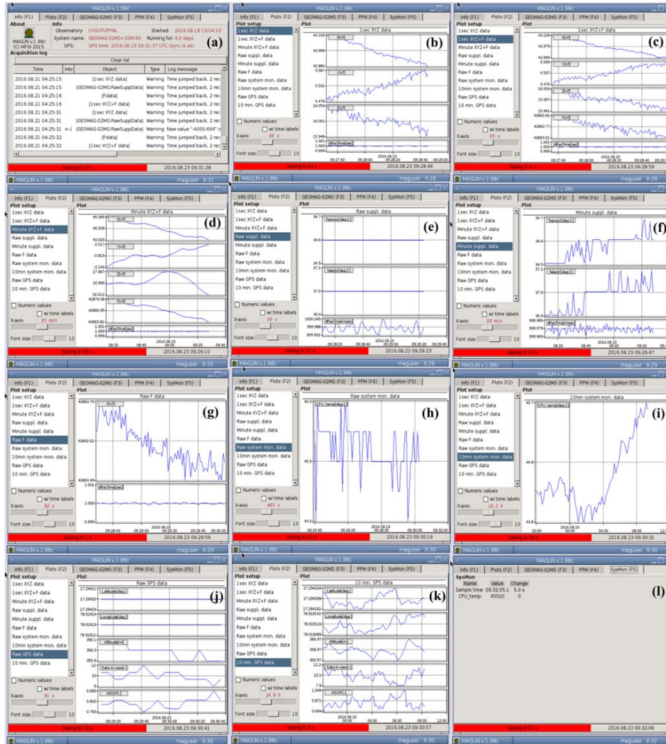
Figure 6: Details of data logging and real-time plotting tools of MAGREC-4B data acquisition system.
