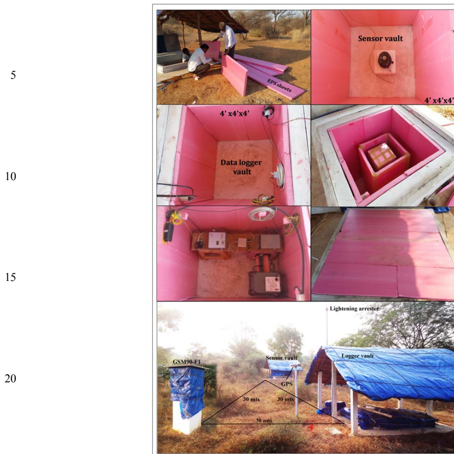
25 Figure 2: Thermally insulated new variometer vaults using Extruded Polystyrene (EPS) foam sheets for good temperature control and the location of sensor and logger vaults.
