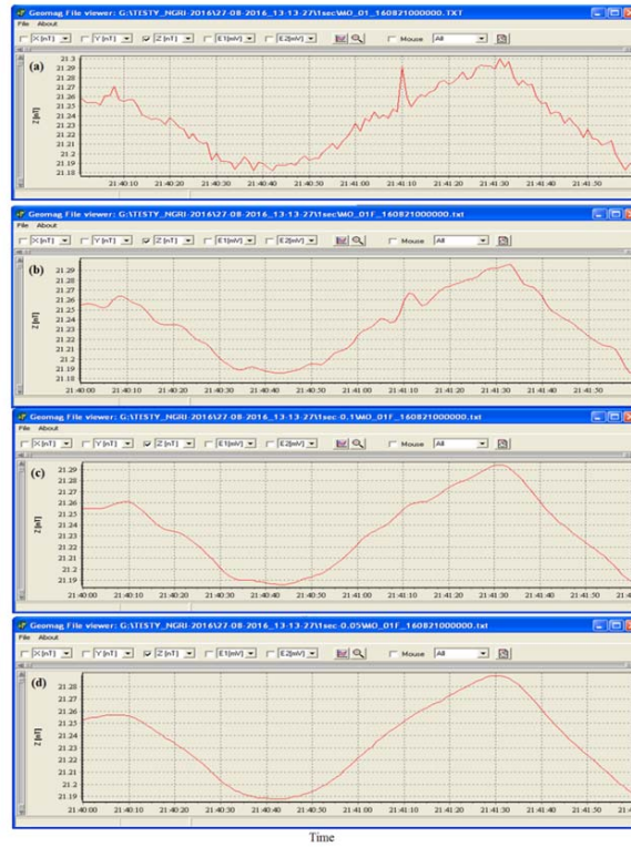
Figure 10: Despiking of data using Low Pass Filter GEOMAG software with different cut-off frequencies.
