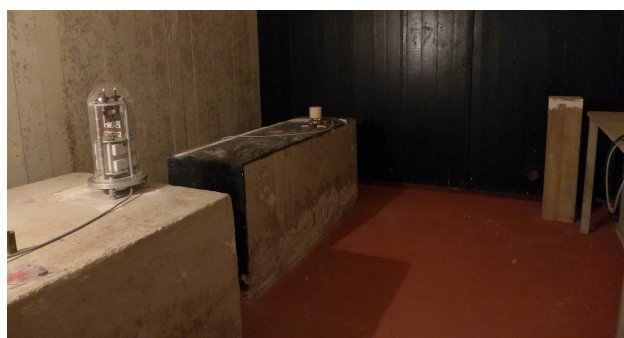
Figure 6. The thermally insulated inner room of the variometer house: The new FGE sensor is placed on the pillar in the front (left), and the LEMI 417 sensor is placed on the pillar in the back. To the right, a part of the shelf with the FGE electronics is visible.
