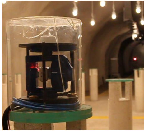
Figure 6. AutoDIF mk2.2 with his plexiglas cloche on pillar A16 in the tunnel of Conrard observatory (WIC).
