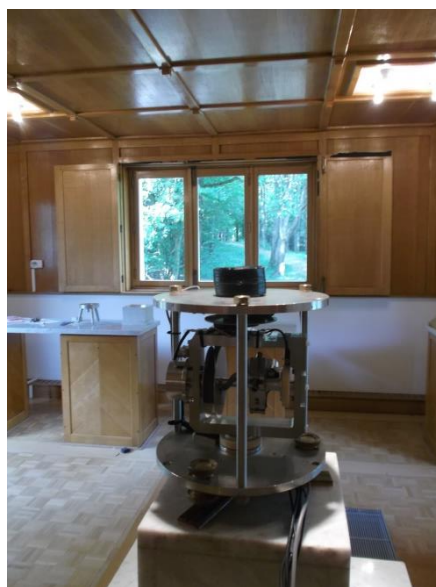
Figure 4. AutoDIF mk2.2 on pillar DO2 in Dourbes absolute house.
