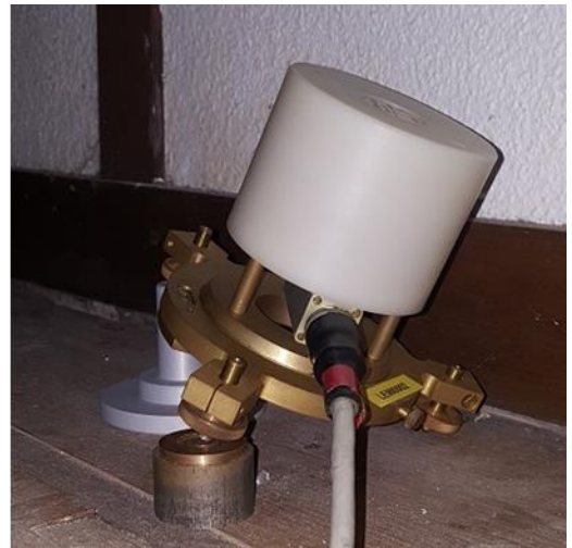
Figure 3: LEMi-025 installed in Dourbes magnetic observatory. The red arrow indicates the True-North direction. The orange arrows highlight the bubble levels saturation.
