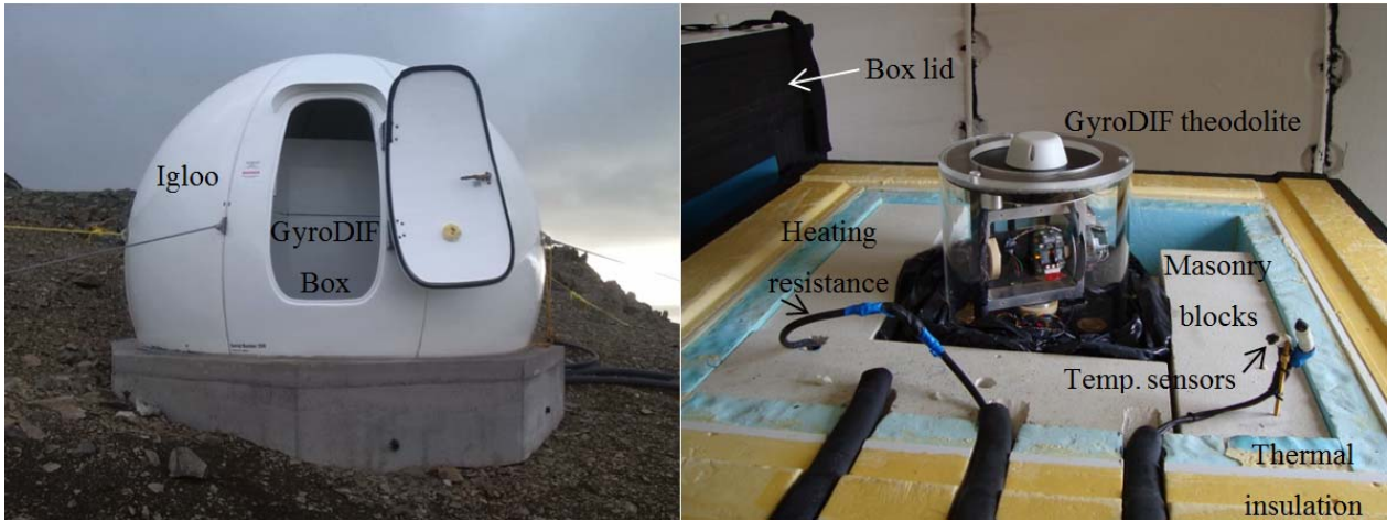
5 Figure 1: Left: Fiberglass igloo and insulating box (interior) for the GyroDIF thermal insulation at LIV. Right: GyroDIF box with lid open inside the igloo; the GyroDIF theodolite is visible in the centre, along with the insulation, the masonry blocks, the temperature sensors and the end of the heating cable.
