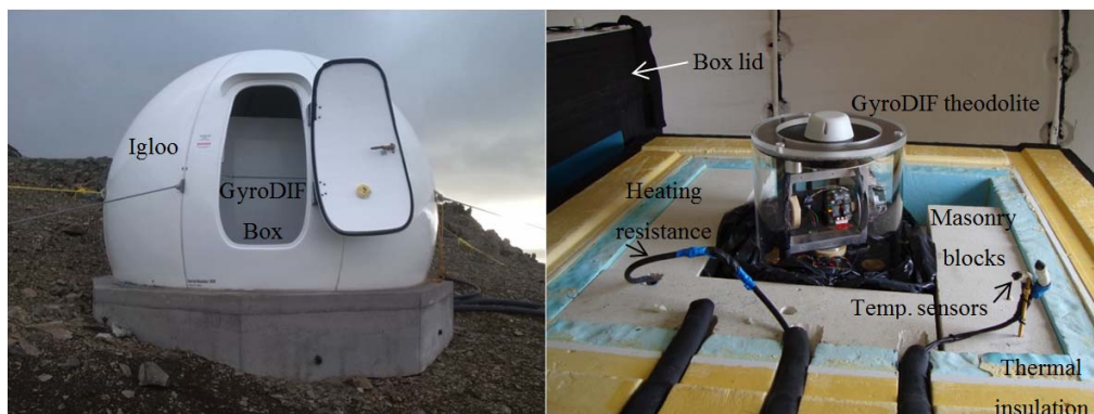
5 Figure 1: Left: Fiberglass igloo and insulating box (interior) for the GyroDIF thermal insulation at LIV. Right: GyroDIF box with lid open inside the igloo; the GyroDIF theodolite is visible in the centre, along with the insulation, the masonry blocks, the temperature sensors and the end of the heating cable.
