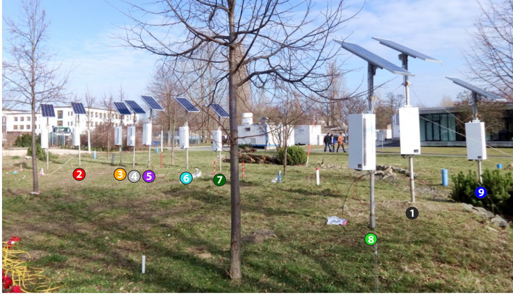
Figure 2. Arrangement of the nine stationary cosmic-ray neutron sensors in the small grass meadow surrounded by highly complex urban terrain.
