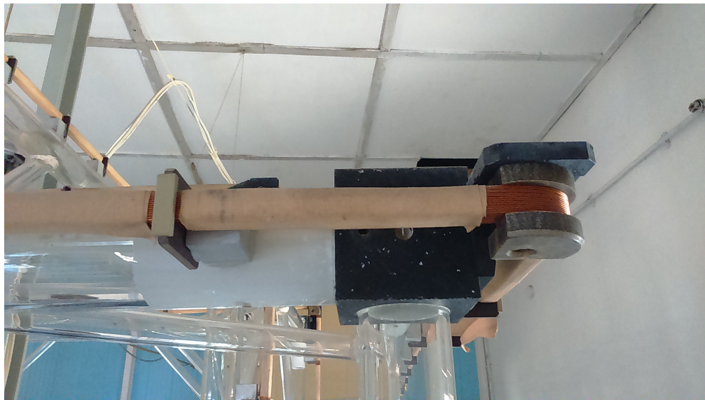
Figure: The Bakelite bracket is used for rolling the coil at the edges and ensures additional stiffness at the edges.
