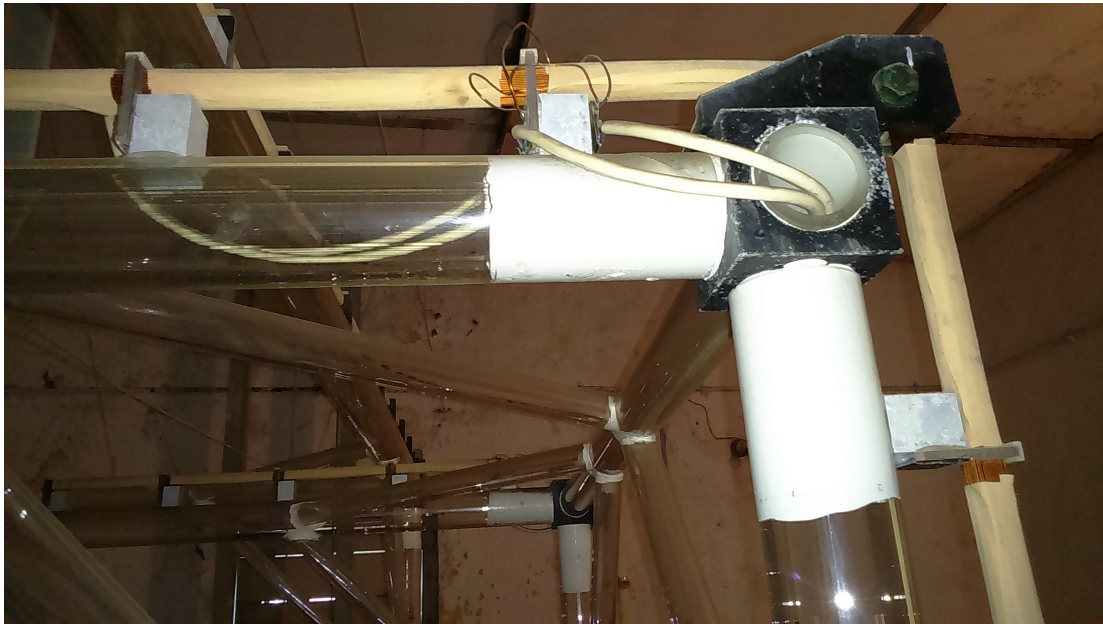
Figure: The coils are supported by a borosilicate glass piping construction to electrically isolate the coils from the support structure. The primary glass support structure at the end corners is joined using a female square design 6 way cross aluminum connector to which a Bakelite bracket is fixed using a nut and a bolt.
