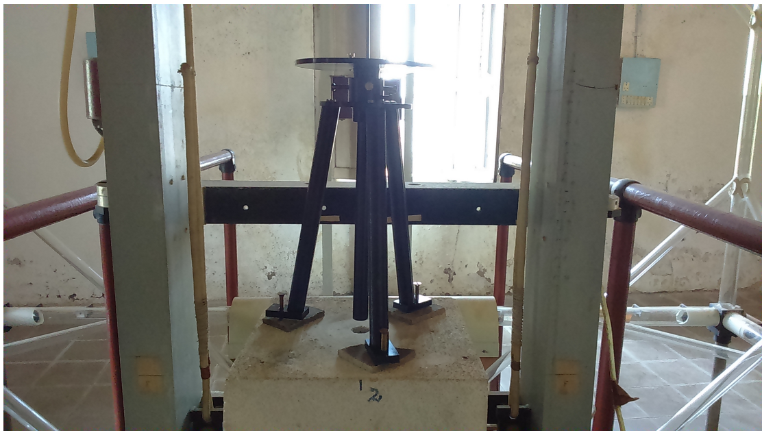
Figure: The sensor to be calibrated is mounted on a non-magnetic table referred to as the test stand which is placed at the centre of the Helmholtz cage.
