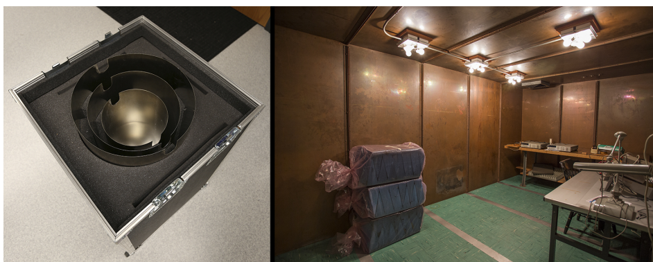
Figure 4. Three-layer shield can (left) and copper room (right) used for the characterization for the PNI RM3100 magnetometer.
