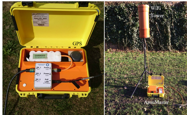
Figure 4. Left: ApsuRx. The break-out-box of ApsuRx provides plugs for three signal inputs, power and WiFi antenna connection. The GPS antenna in the top-right corner is used for time synchronization. Right: ApsuMaster is connected to the WiFi tower which consists of a array of WiFi antennas working in the AP mode.
