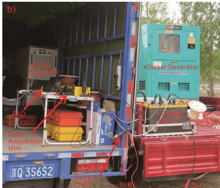
Figure 1. a) Diagram of multifunction EM transmitter architecture, b) picture of the transmitter (diesel generator, AC/DC regulator chopper module, current probe, data acquisition unit, cable, tablet computer (PAD))
