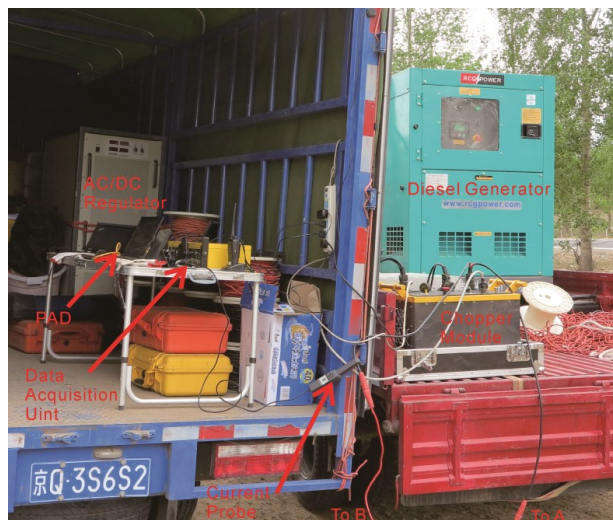
Figure 1. Diagram of multifunction EM transmitter architecture (diesel generator, AC/DC regulator chopper module, current probe, data acquisition unit, cable, tablet computer (PAD))
