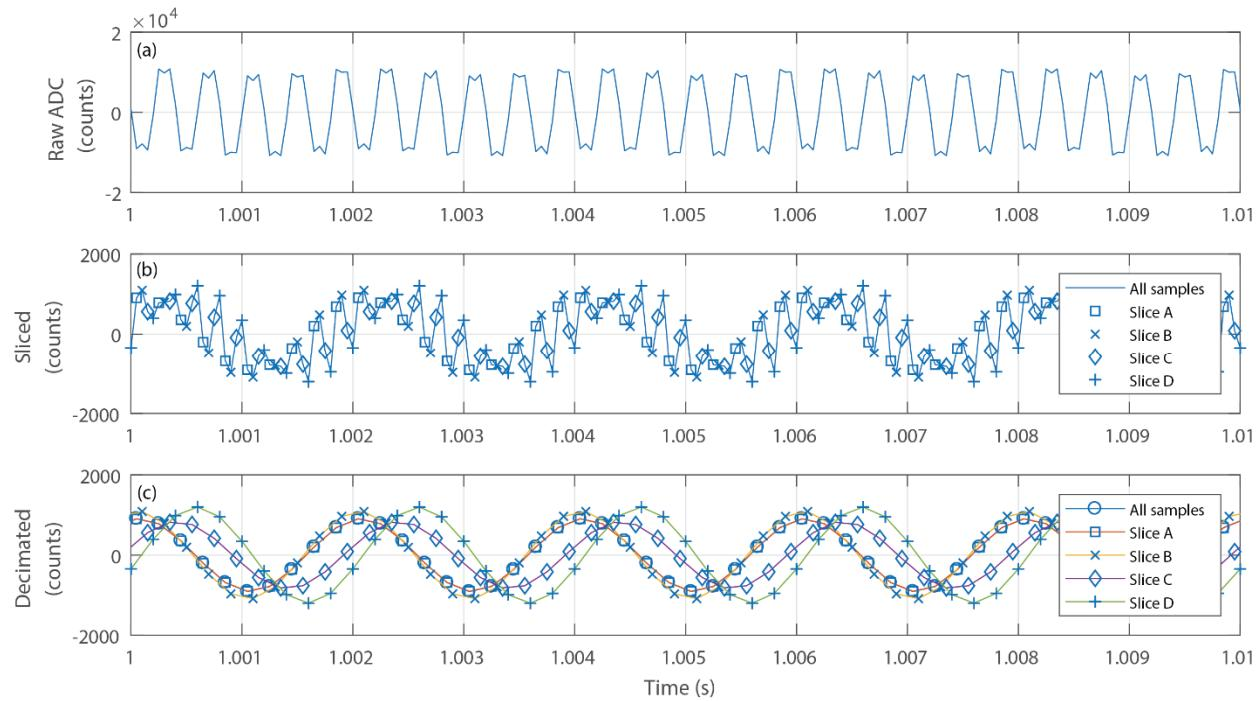
At 500 Hz the reconstructions from all data and from the four slices are more in phase and show variation in gain consistent with various states of core saturation. We suspect that this data is still somewhat contaminated with residual aliased fluxgate signal. However, at higher frequencies the coil response dominates which will also mask the effect of core saturation. The 500 Hz test signal was taken as the best compromise available from the current data showing the effect of core saturation.
