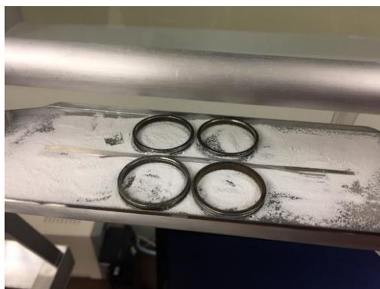
**Figure 13: Ring-cores on a molybdenum loading-plate in a loading chamber. Alumina powder prevented the ring-cores from welding to the plate.**
