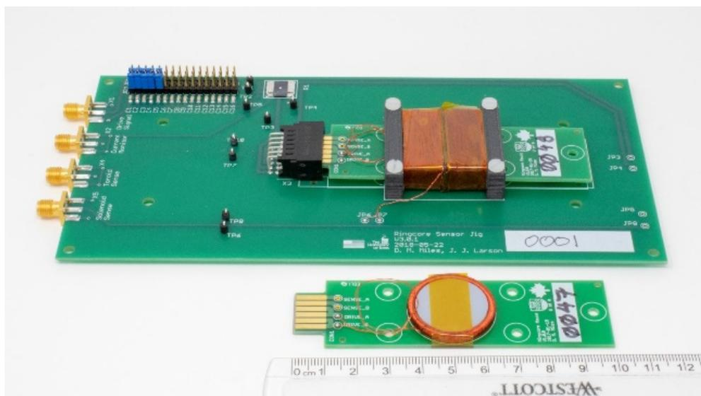
**Figure 16: Test jig used to rapidly characterize multiple ring-cores. Each ring-core has a toroidal drive winding applied and is mounted on a small printed circuit board. The mounted ring-core inserts through a modified sense winding and the entire assembly is placed in a solenoid/magnetic shield for testing.**
