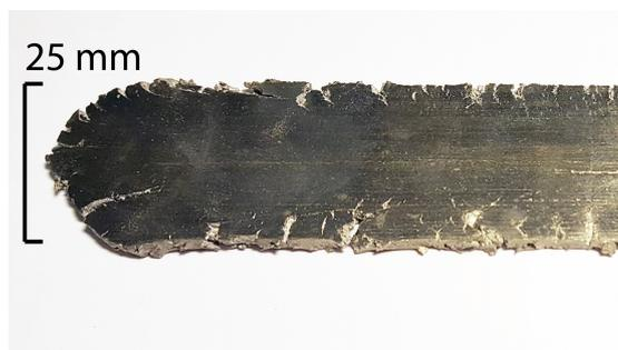
**Figure 6: 3 mm thick stock machined from the 6-81 permalloy ingot showing the surface cracking that resulted from an attempt at hot-rolling.**
