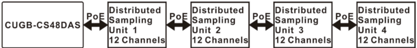
Figure 7: Distributed and centralized seismograph.
