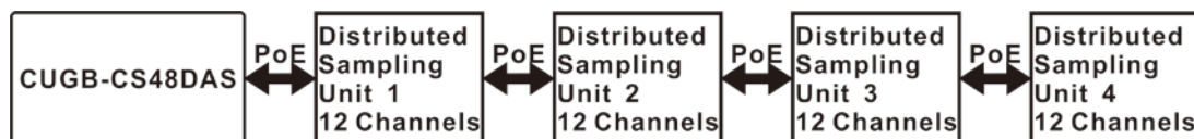
Figure 7: Distributed and centralized seismograph
