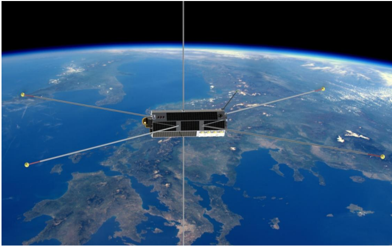
Figure 12: Spacecraft observation geometry: Daedalus s/c with extended field booms; four electric field booms are arranged in X-formation in the along-cross-track plane and two booms are aligned vertically (left). Ram direction instrumentation (right).
