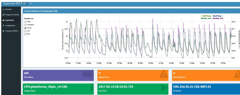
5 Figure 11: Screenshots of the “supervision menu” of the user interface. A time series graph is displayed with minimum and maximum battery voltage on the 1st y-axis, min and max air temperature on the 2nd y-axis
