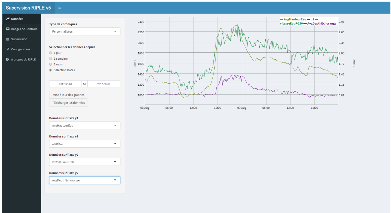
5 Figure 9: Screenshot of the “data visualization menu” of the user interface in the personalized mode. A graph can be created with two variables on the 1st y-axis, two variables on the 2nd y-axis and in abscissa the time. In this case, the water level, water surface velocity and distance measured by the echo sounder are displayed.
