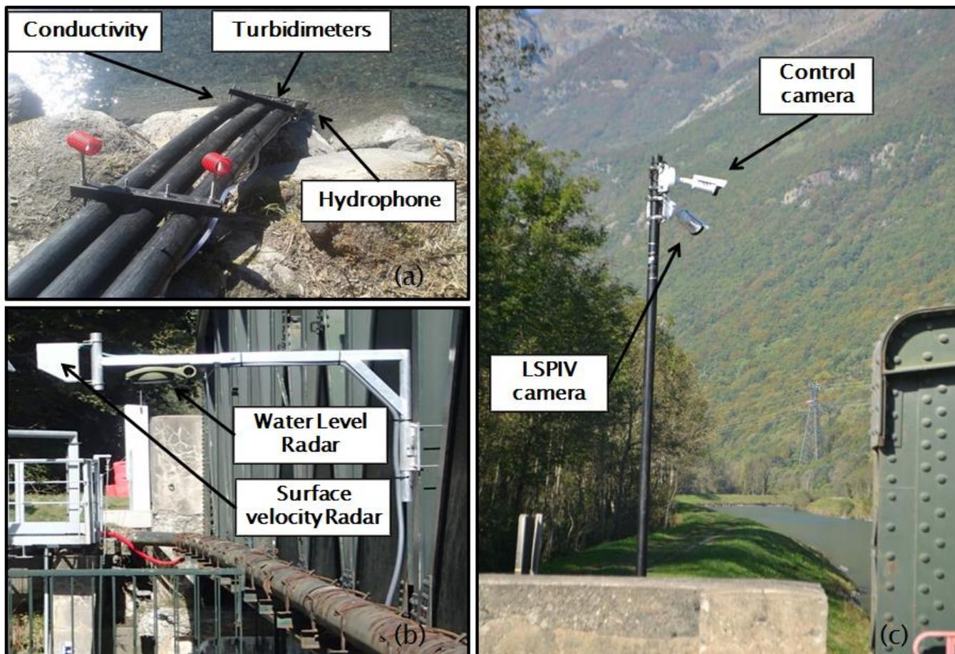
5 **Figure 4: Photos illustrating the deployment of instruments in situ (a) submerged instruments (conductivity probe, turbidimeters and hydrophone) housed in the polypropylene tubes anchored to the river bank, (b) water level and surface velocity radars supported by extensible brackets fixed to the bridge parapet, (c) control digital camera and LSPIV digital camera fixed at the top of a mast located on a river bank.**
