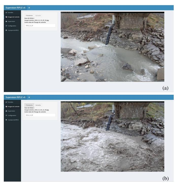
Figure 10: Screenshots of the "images of control menu" of the user interface at two dates: (a) 06/11/2018 12:00 (UTC) for low water conditions, (b) 19/12/2018 10:00 (UTC) during a flood
