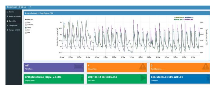
Figure 11: Screenshots of the "supervision menu" of the user interface. A time series graph is displayed with minimum and maximum battery voltage on the 1st y-axis, min and max air temperature on the 2nd y-axis
