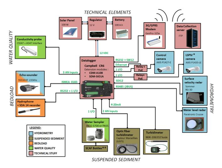
\* LSPIV : Large Scale Particle Image Velocimetry
