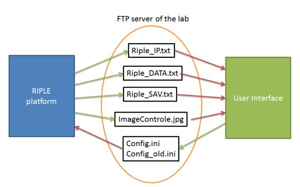
Figure 6: Diagram describing the links between the RIPLE platform, the remote server and the user interface
