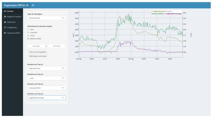
Figure 9: Screenshot of the "data visualization menu" of the user interface in the personalized mode. A graph can be created with two variables on the 1st y-axis, two variables on the 2nd y-axis and in abscissa the time. In this case, the water level, water surface velocity and distance measured by the echo sounder are displayed.
