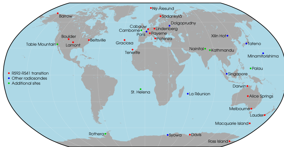
Fig. 1. Locations of GRUAN sites and other transition-related sites (September 2019). Red dots represent sites that switched from RS92 to RS41 as their operational radiosonde. Blue dots represent sites that employ another type of radiosonde or that transitioned from another type to the RS41. Green dots represent sites which performed additional comparison launches and provided these data to GRUAN.
