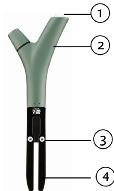
Figure 1. Schematic of the FP sensor: 1. light intensity, 2. ambient temperature, 3. fertilizer level, and 4. soil moisture sensor (Parrot, 2019d).
