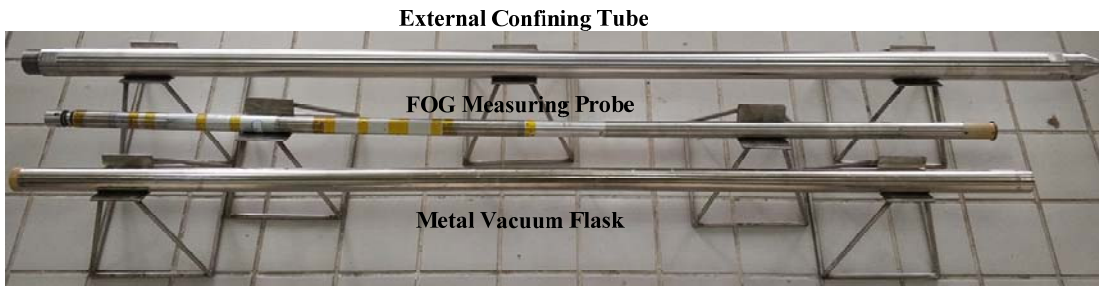
85 Figure 2: Photos of external confining tube, metal vacuum flask, and FOG measurement probe.
