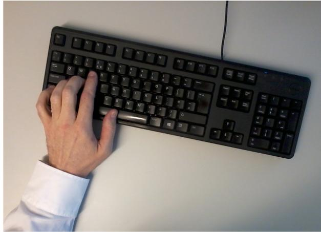
**Figure 4.** Hand position for the left-key set, with the keyboard at an angle of 10–15 degrees, to minimise finger reach strain.
