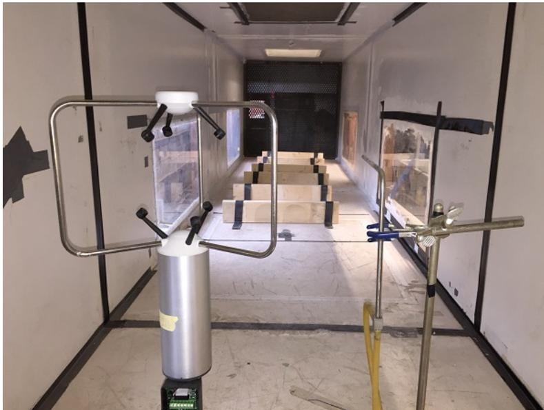
Figure 5: The view of the R.M. YOUNG 81000 (left) and pitot tube (right) at the wind tunnel.
