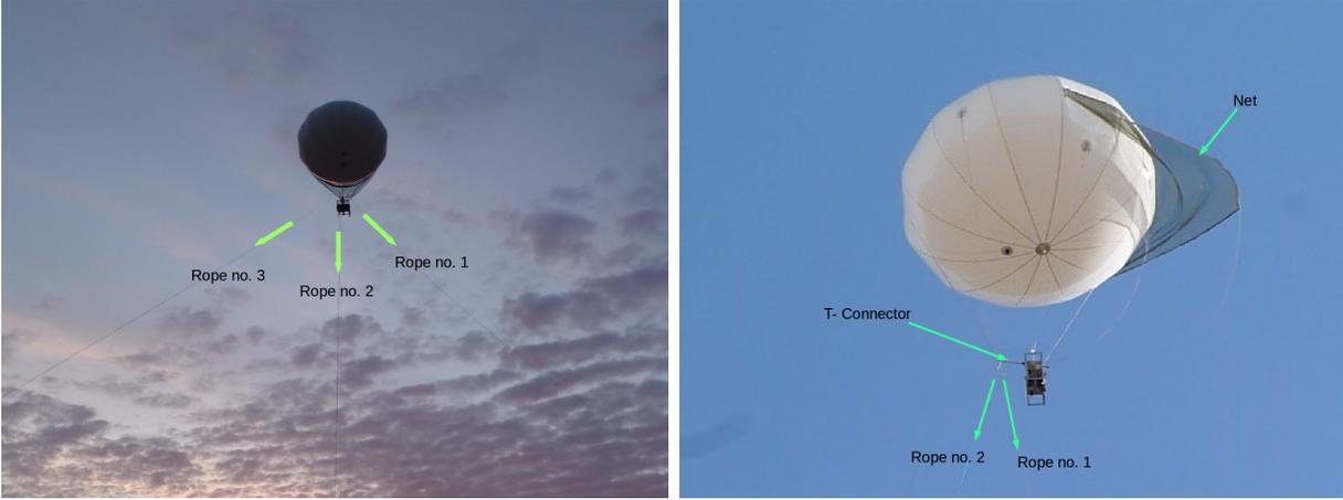
Figure 2: TANAB at different atmospheric stability conditions; left: TANAB and three stabilizing ropes deployed at the mining facility; right: TANAB and two stabilizing ropes deployed at the mining facility.
