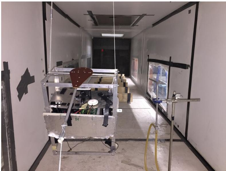
Figure 6: The view of gondola (left) and pitot tube (right) at the wind tunnel.
