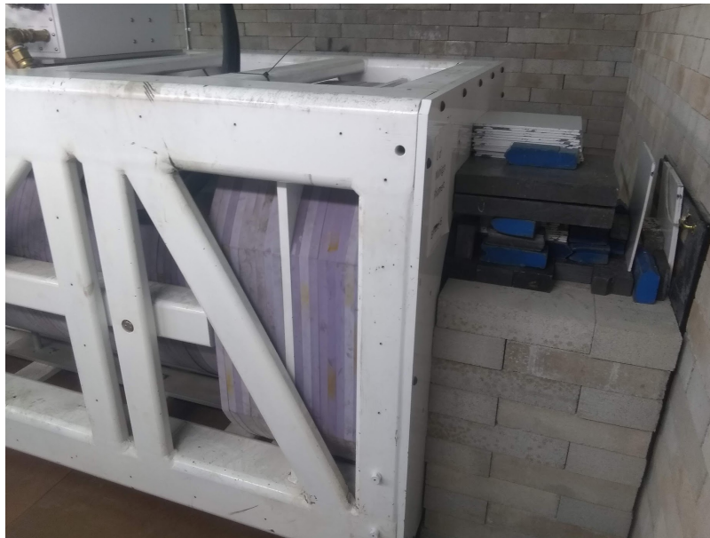
Figure 4. Detail of the output end of the Varian M9 linear accelerator at the Department of Nuclear Engineering and Radiological Sciences at the University of Michigan. The exit of the beam is located at the right hand side of the figure, and the magnetometer being irradiated is located behind the wall on the right.
