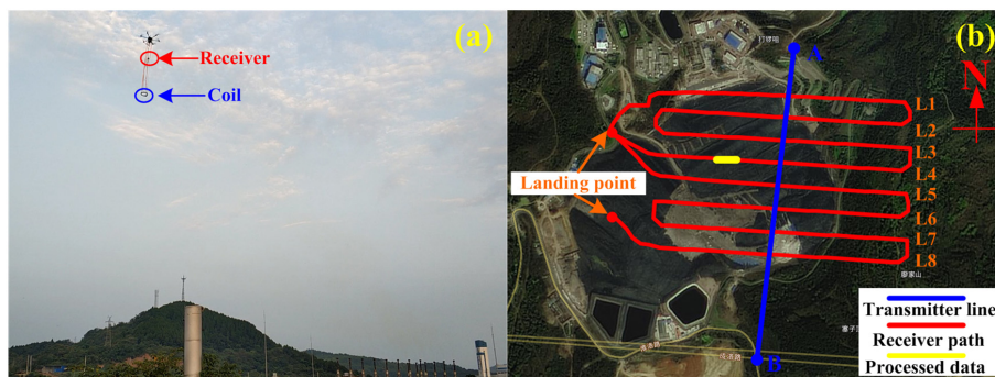
305 Figure 5: The survey area and flight paths of the GREATEM system. (a) The receiver system is mounted on UAV along the paths. (b) The blue line was the transmitter source and the red line was the survey path of the receiver. The flight heading was from east to west on the L4 path. The data of part of L4 (yellow solid line) was processed and the length of time was 60 seconds. (b) embedded the satellite images came from https://map.tianditu.gov.cn/ , built by the National Geomatics Center of China.
