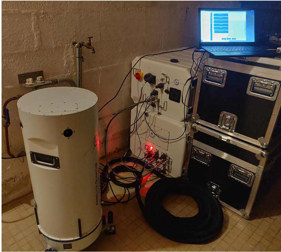
Figure 1. AQG-B01 in a garage in Montpellier in June 2020. The sensor head (left) is connected with the laser- and electronic systems by 5 m of cables. The AQG GUI software is used on a laptop to control the measurement as well as to correct, visualise and analyse the gravity data.
