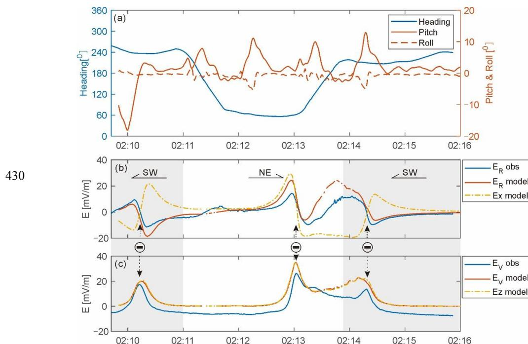
431 **Figure.6.** Comparison of the measured data and numerical simulation. (a) Navigation attitude of AUV
