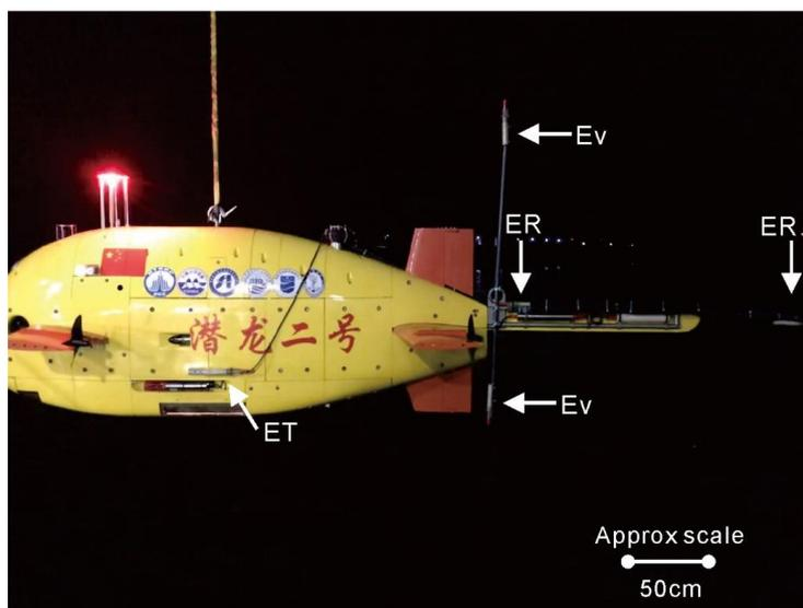
399 **Figure.1.** Layout of each channel electrode on AUV.  $E_R$  is the inline horizontal component of electric
