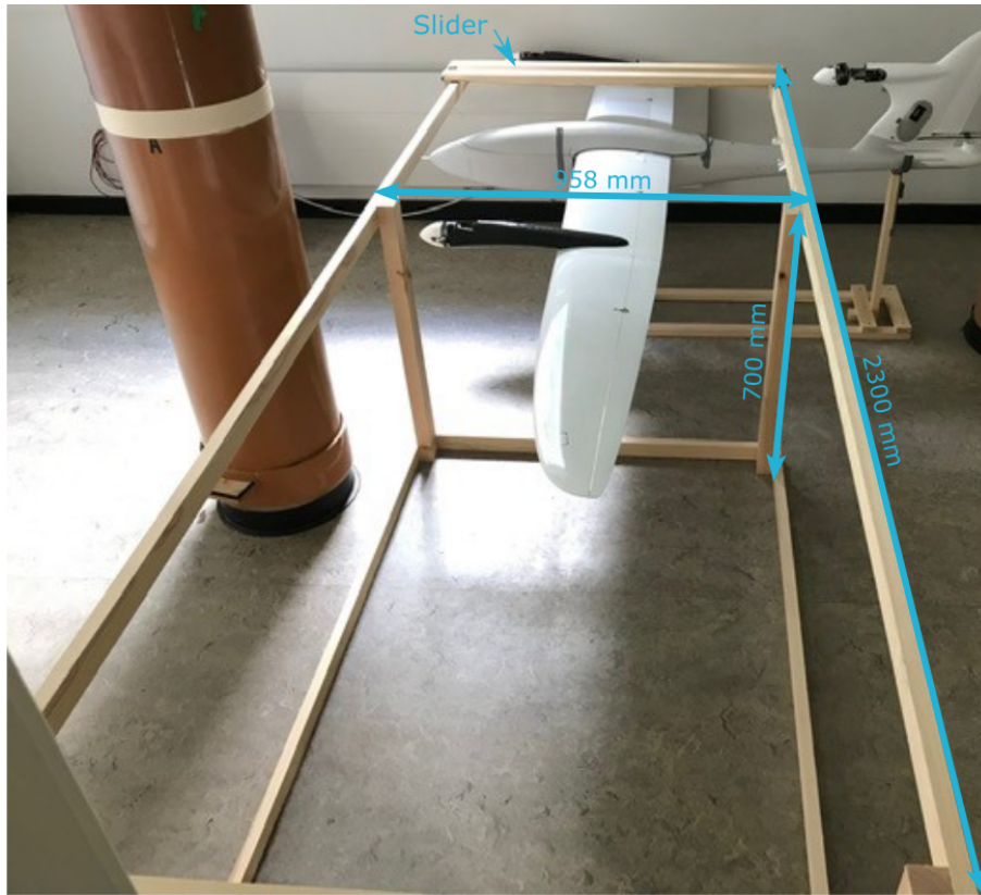
Figure 2. Demonstration of the magnetic signature measurement of the port wing. The length and the width of the slider are 1000 and 150 mm, respectively.
