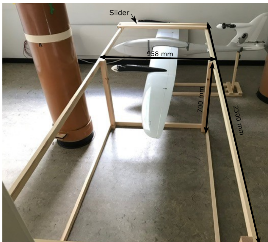
Figure 1. Demonstration of the magnetic signature measurement of the port wing. The length and width of the slider are 1000 and 150 mm, respectively.
