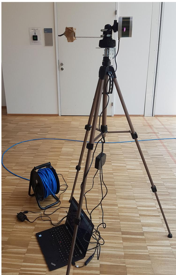
**Figure 2.** Terrestrial lidar system (TLS)
