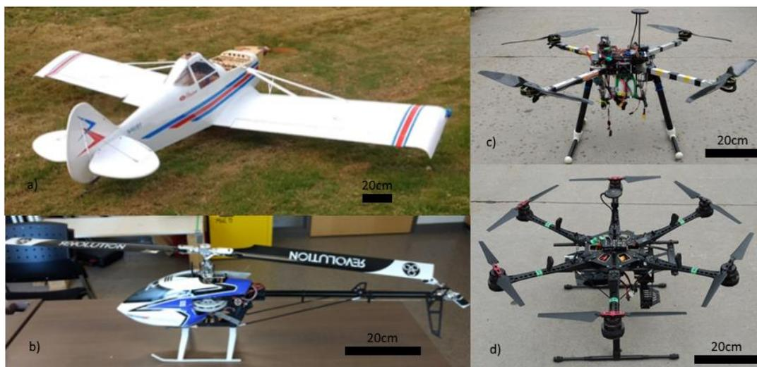
430 **Figure 1:** Photographs of the UAS investigated in this study. a) single-motor fixed-wing, b) single-rotor helicopter c) quad-rotor helicopter, and d) hexa-rotor helicopter.
