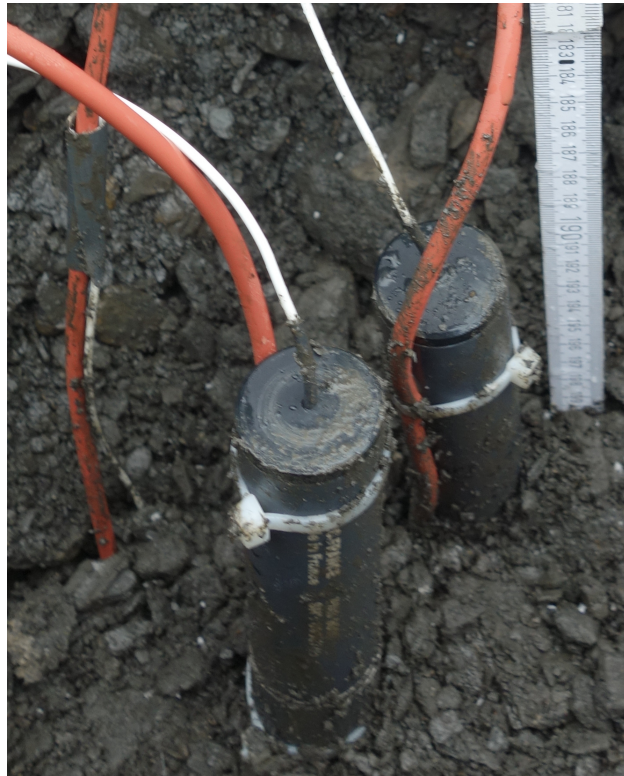
Figure 3. Installation of electrodes 1 and 19. Electrode 20 is located directly below these both electrodes, indicated by the feeding cables on the left. White cables are connected to the electrodes, while red cables house four stranded wires leading to Pt100-temperature sensors at the tip of each electrode.
