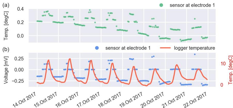
**Figure 11.** a) Temperature curve for sensor at electrodes and 5. b) Corresponding voltages (blue), measured over the Pt100 resistance of the temperature sensor before current injection, and logger temperature (red).
