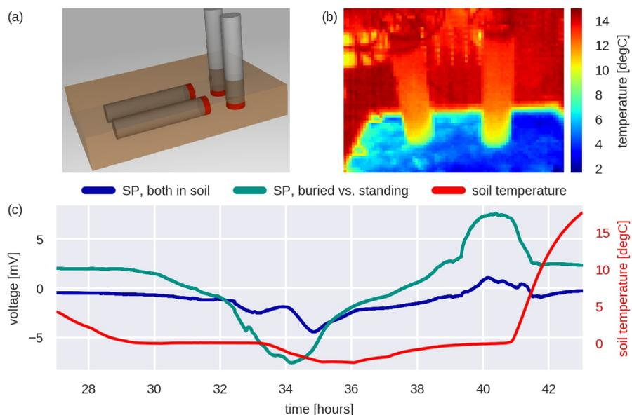
**Figure 7.** Laboratory experiment investigating electrode effects during freezing and thawing. a) Sketch of experimental setup. The container is 30 cm in length, 20 cm in depth, and 5 cm high. Electrodes are shown in gray, with the wood membranes in contact with the surrounding highlighted in red. b) Thermal image (surface temperatures) during thawing c) Electrical voltages and soil temperatures; vertical black line indicates time of thermal image in b)
