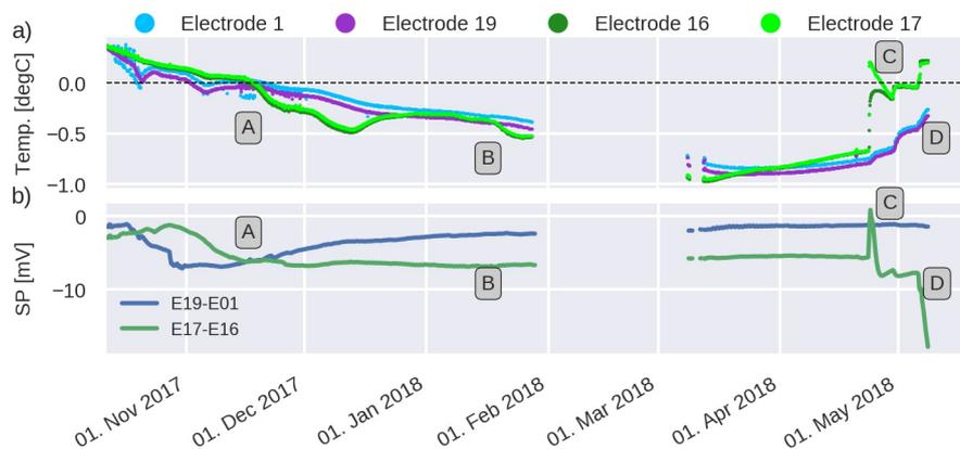
**Figure 13.** Measured voltages between references electrodes 1 and 16 and their respective duplicated electrode, located a few cm away. a) Temperature readings of all four involved electrodes. b) Voltage readings between duplicated electrodes 1 and 19, and 16 and 17.
