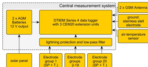
**Figure 4.** Schematic overview of essential system components. Components included in the group "Central measurement system" are housed in an aluminium box (see also Fig. 5), while all other components are external and connected by cables. The term 'electrode group' refers to each pair of SP-electrode and attached temperature sensor. The components termed 'lightning protection and low-pass filter' were only installed and tested in 2019.
