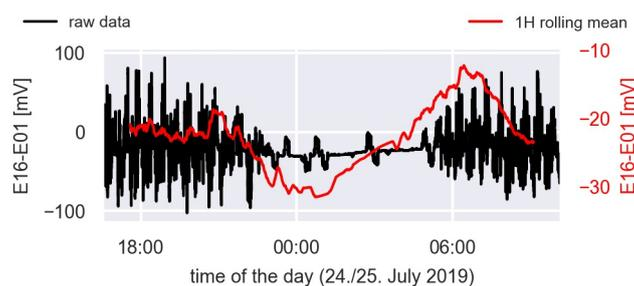
**Figure 8.** Noise measurement on dipole E16-E01, conducted in the summer of 2019. Raw data is drawn in black, a 2 hour moving average filtered version in red.
