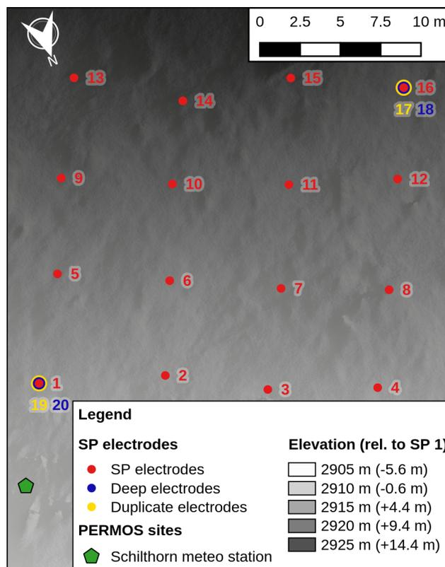
**Figure 2.** Electrode layout at the Schilthorn summit. Electrodes are roughly 7.5 m apart in horizontal and vertical directions. Deep electrodes 18 and 20 are located 20-30 cm below the reference electrodes 1 and 16, respectively, while electrodes 17 and 19 duplicate the reference electrodes 1 and 16, respectively, in only a few cm distance (see Fig. 3 for photograph of electrodes 1 and 19). The legend denotes absolute electrodes heights, as well as heights relative to electrode one.
