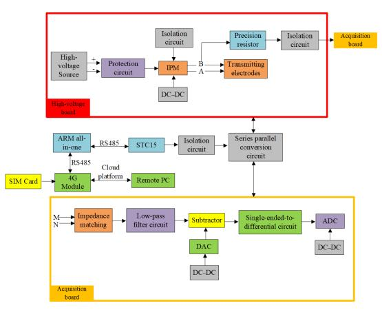
95 Figure 3: High-level architecture of the 4D high-density electrical instrument based on IoT.
