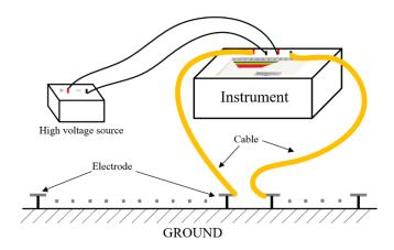
Figure 2: Principle of the high-density electrical method.
