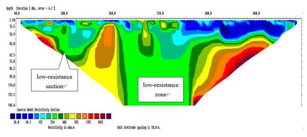
Figure 15: Profile view of Survey Line L1 obtained using the high-density electrical method.
