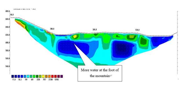
255 Figure 16: Profile view of Survey Line L2 obtained using the high-density electrical method.
