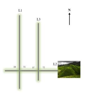
Figure 13: Schematic layout of the survey lines. (The 75th measurement point on the L1 survey line intersects with the 59th measurement point on the L2 survey line, and the 72nd measurement point on the L3 survey line intersects with the 57th measurement point on the L2 survey line.)
