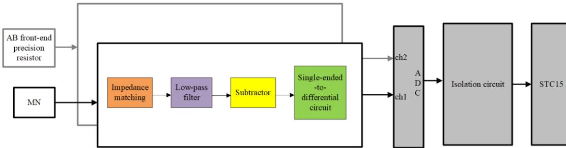
Figure 4: Block diagram of the AB.
