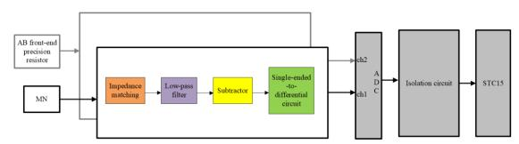
Figure 4: Block diagram of the AB.
