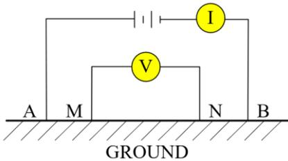
**Figure 1: Principle of the basic electrical method.**
