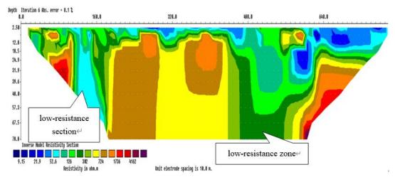
Figure 17: Profile view of Survey Line L3 obtained using the high-density electrical method.
