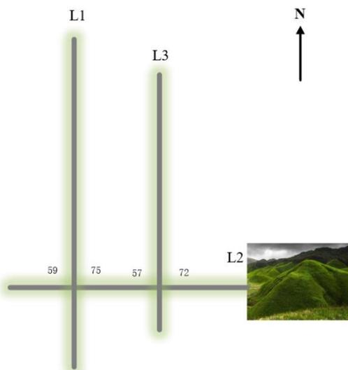
225 **Figure 13: Schematic layout of the survey lines. (The 75th measurement point on the L1 survey line intersects with the 59th measurement point on the L2 survey line, and the 72nd measurement point on the L3 survey line intersects with the 57th measurement point on the L2 survey line.)**
