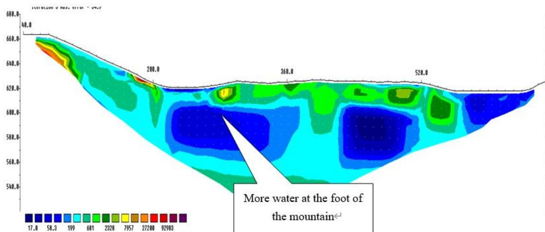
255 **Figure 16: Profile view of Survey Line L2 obtained using the high-density electrical method.**
