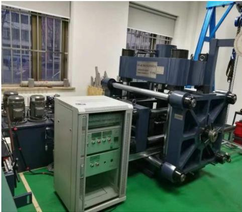
(c) rock true triaxial testing machine
