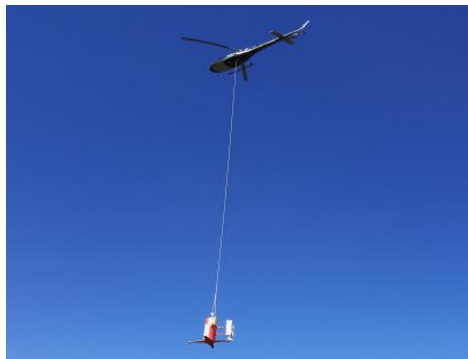
Figure 1: Towed bird system
