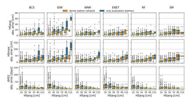
**Figure 5.** Boxplots of absolute errors in average snow depth in a winter (HSavg, top row), maximum snow depth in a winter (HSmax, middle row) and number of snow days with HS $\geq$ 1 cm (dHS1, bottom row) calculated for 20 cm HSavg bins of the respective gap-winter and the different methods (columns) respectively. Colors of the boxplots denote the different station networks that have been used for reconstruction. Outliers in the boxplots are not shown for better comparison.
