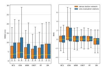
**Figure A2.** Boxplots for root-mean-squared error (RMSE) and BIAS of the daily values for the different methods and station densities. The maximum number of predictors for the different methods is set as defined in Tab. 1. The station network density is irrelevant for the snow model as no data from neighboring stations is used. For better comparison, outliers are not shown in the boxplots.
