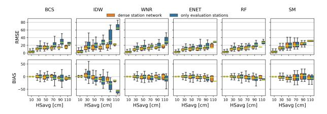
**Figure A1.** Boxplots of RMSE (top row) and BIAS (bottom row) calculated for 20 cm HSavg bins of the respective gap-winter and the different methods (columns) respectively. Colors of the boxplots denote the different station networks that have been used for reconstruction. Outliers in the boxplots are not shown for better comparison. The maximum number of predictors for the different methods is set as defined in Tab. 1.
