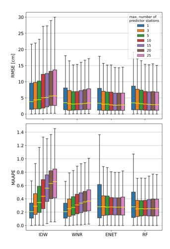
**Figure 2.** Boxplots of RMSE and MAAPE calculated in the individual reconstructed winters with varied maximum number of predictor stations for the spatial interpolation methods. The methods have been applied to the complete station network. For better comparison, outliers are not shown in the boxplots. Note that WNR with one predictor station is equivalent to the BCS method.
