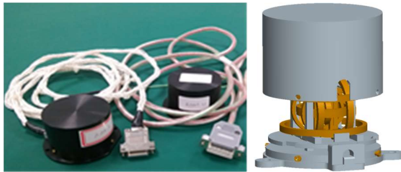
Figure 2: (a) The real sensor picture and (b) the structure design diagram of the sensor.
