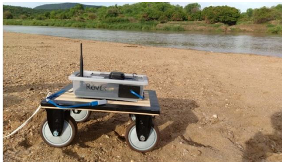
Figure 5 (a) Low Cost RTK GNSS Rover mounted on a mobile cart for recording RTK water line 5 (b) ADCP combined with an RTK GNSS Rover attached to a fisherman's canoe measuring the wet bathymetry.
