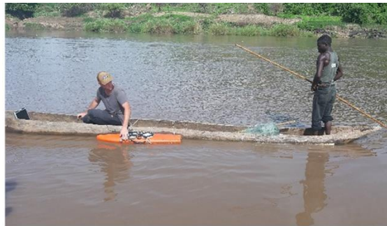
Figure 5 (a) Low Cost RTK GNSS Rover mounted on a mobile cart for recording RTK water line 5 (b) ADCP combined with an RTK GNSS Rover attached to a fisherman's canoe measuring the wet bathymetry.
