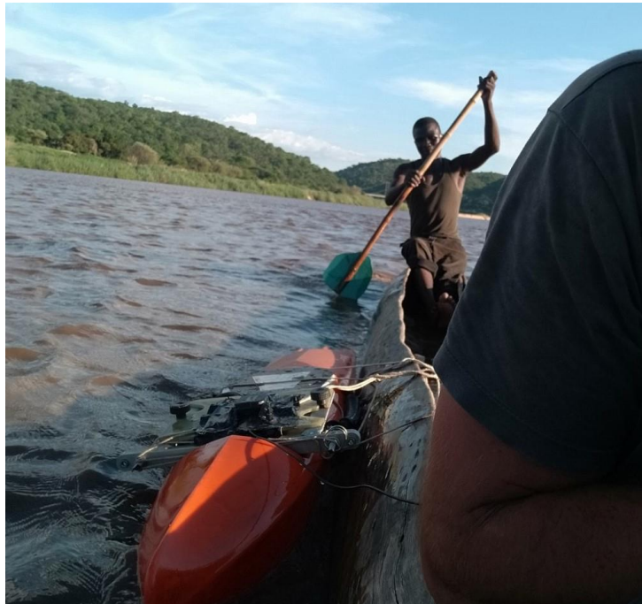
Fig. A2. ADCP with a Low cost RTK GNSS attached to canoe
