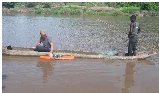
275 Figure 5 (a) Low Cost RTK GNSS Rover mounted on a mobile cart for recording RTK water line 5 (b) ADCP combined with an RTK GNSS Rover attached to a fisherman's canoe measuring the wet bathymetry.
