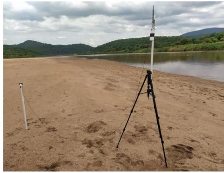
220 Figure 2 (a) RTK GNSS Set (b) RTK GNSS Base Station Setup along the Luangwa River Floodplain
