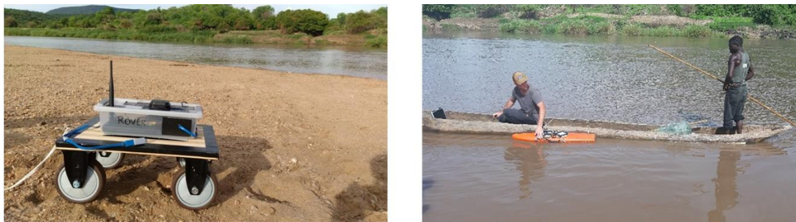
Figure 5 (a) Low Cost RTK GNSS Rover mounted on a mobile cart for recording RTK water line 5 (b) ADCP combined with an RTK GNSS Rover attached to a fisherman's canoe measuring the wet bathymetry.
