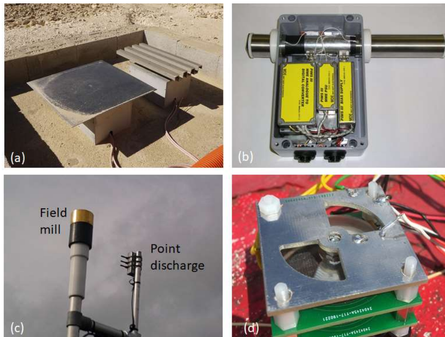
Figure 3 A selection of atmospheric electricity instruments. (a) Vertical current density sensor (GDACCS), using plate and corrugated electrodes, in the Negev desert. (b) Programmable Ion Mobility Spectrometer (PIMS) to determine electrical properties of air. (c) Electric field mill with sensing surfaces uppermost, and upward pointing point discharge needle (not visible) with logarithmic current amplifier. (d) Miniature field mill with internal calibration electrodes.
