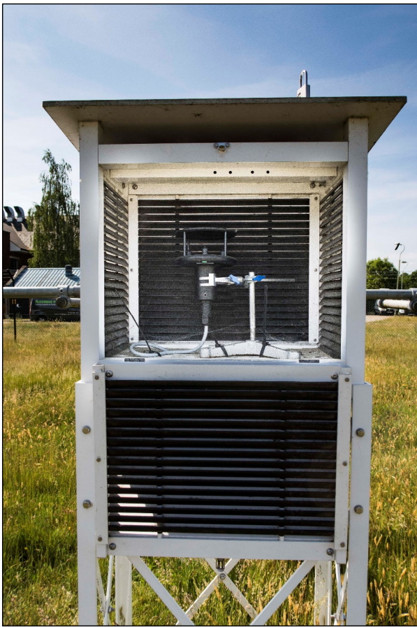
Fig. 2. The Gill Windsonic anemometer secured within the Stevenson screen shown in Figure 1. The inside dimensions of the screen were 50 cm width x 25 cm depth x 43 cm height. This photograph was taken on 27 May 2020. Photograph © Copyright Stephen Burt
