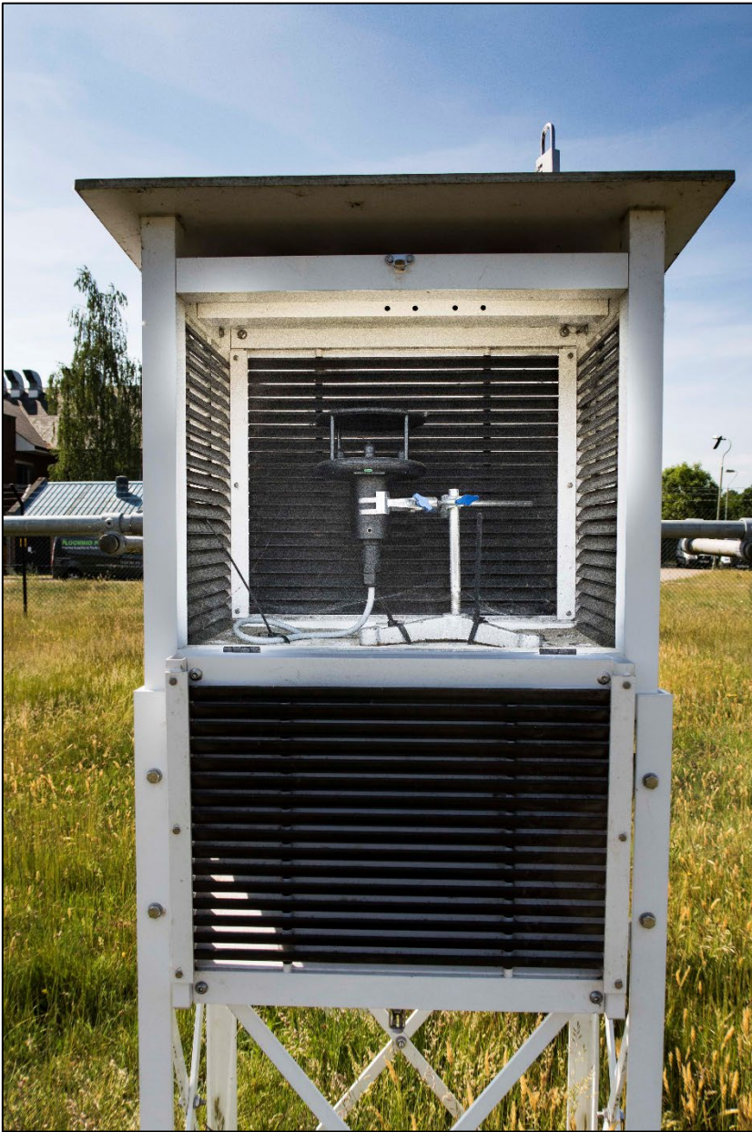
Figure 2. The Gill Windsonic anemometer located within the Stevenson screen shown in Figure 1. The inside dimensions of the screen were 50 cm width x 25 cm depth x 43 cm height. This photograph was taken on 27 May 2020. Photograph © Copyright Stephen Burt
