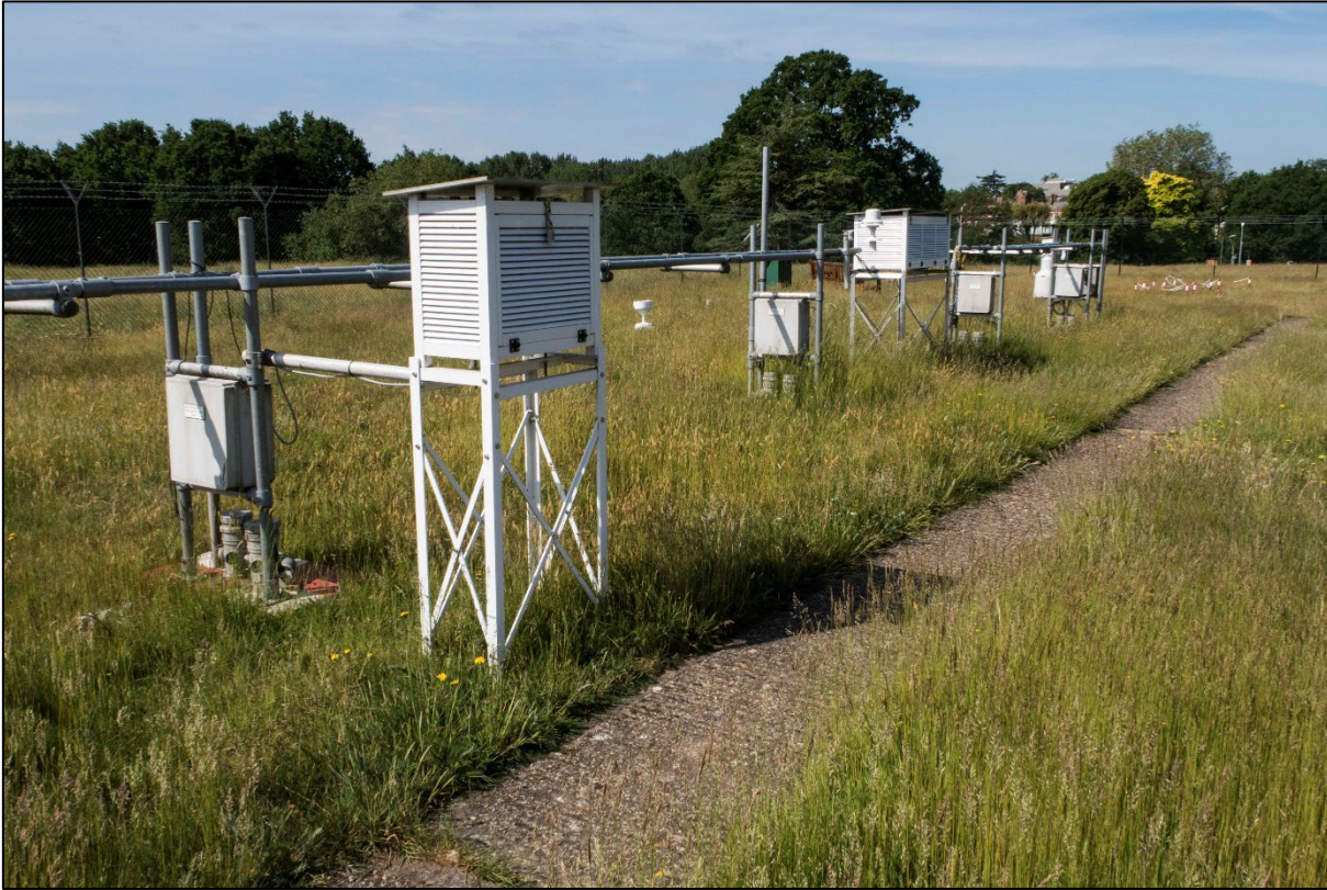
435 Figure 1. Within the Reading University Atmospheric Observatory enclosure: the screen nearest to the camera housed the Gill Windsonic anemometer used in this experiment, and its screen door (shown with padlock) opens to true North. This photograph was taken on 27 May 2020. Owing to the coronavirus emergency legislation, the university campus had been closed for two months at this time and normal grass cutting and maintenance work suspended. Photograph © Copyright Stephen Burt
