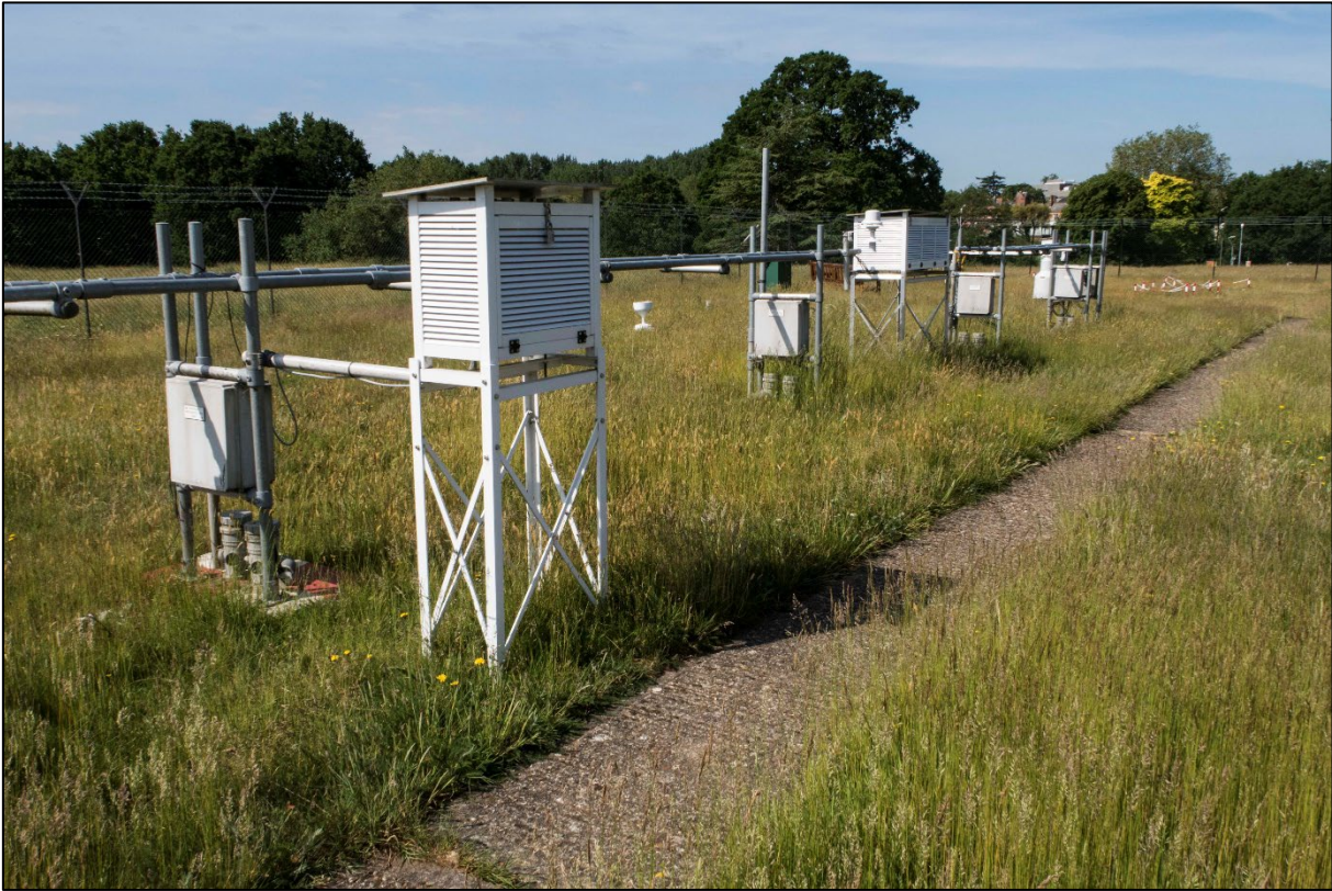
Figure 1. Within the Reading University Atmospheric Observatory enclosure: the screen nearest to the camera housed the Gill Windsonic anemometer used in this experiment, and its screen door (shown with padlock) opens to true North. This photograph was taken on 27 May 2020. Owing to the coronavirus emergency legislation, the university campus had been closed for two months at this time and normal grass cutting and maintenance work suspended. Photograph © Copyright Stephen Burt
