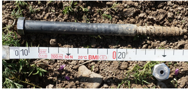
Figure 3. Stainless-steel electrode used for sEIT measurements. Scale is in cm.
